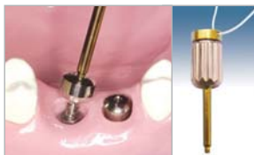
Left : Separating the healing abutment using a driver Right : Hand driver with dental floss tied to the handle
