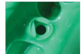
The triangle circle structure replicated on the coping
