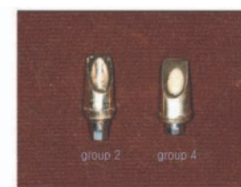
Fig. 4. UCLA-type abutments after casting procedure (group 2: internal hexagonal implant, group 4: internal octagonal implant).
