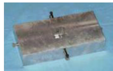
Fig 1. Aluminum block for stabilizing bone specimen.
