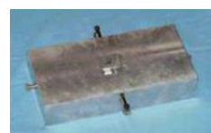
Fig 1. Aluminum block for stabilizing bone specimen.
