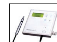
Periotest ® Damping capacity assessment
