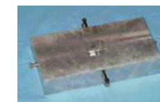
Fig 1. Aluminum block for stabilizing bone specimen.
