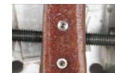
Fig 2. Bone specimen fixed in aluminum block.
