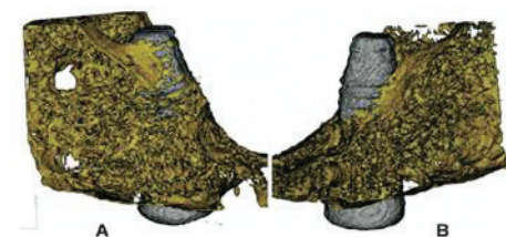
Fig 3. Three-dimensional microCT showing the bone (yellow) around implants (gray). A, Corticocancellous block bone graft. B, Corticocancellous particulate bone graft.
