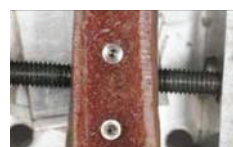
Fig 2. Bone specimen fixed in aluminum block.
