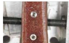
Fig 2. Bone specimen fixed in aluminum block.
